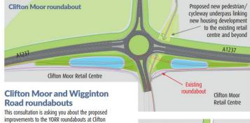
The blueprint for improving the capacity at all the roundabouts is based on providing three lane entries on the Ring Road approaches to the roundabout and two lane exits. This will provide an increase in the junction capacity similar to those implemented at the AS9. A19 and Wetherby Road roundabouts.
